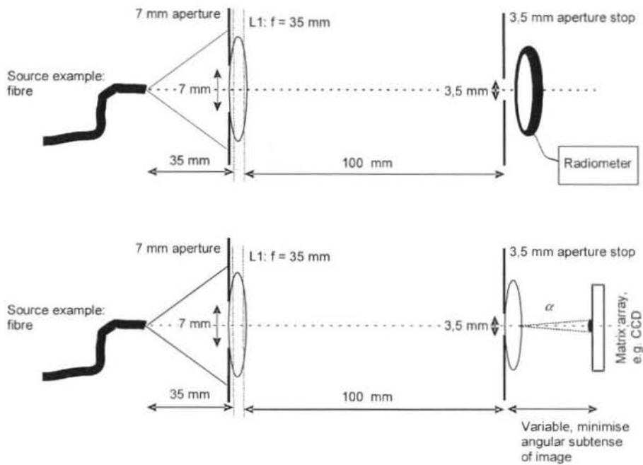
Figure 3: Set-up for Condition 2 according to IEC 60825-1, ed.2 (2007).
