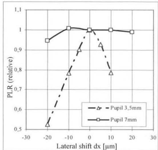
Figure 2: PLR (relative) as a function of the lateral shift  $dx$  of the loupe for two pupil diameters. Light source: diode laser,  $\lambda=660$  nm, fiber 125/50, measurement set up according to figure 5 but the focal length was changed:  $f_L=15$  mm (magnification 17), distance fiber end to loupe = 13 mm.
