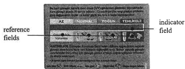
Figure 1. Example of a UV irradiance indicator card with indication of the indicator field and the reference fields.
