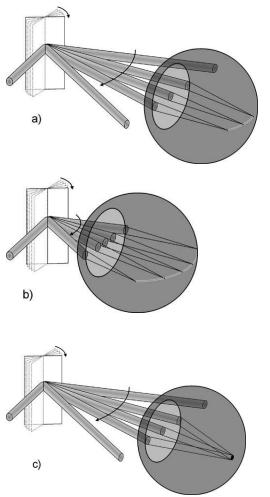
**Figure 1.** For a well collimated beam that is scanned across the pupil of the eye, if the eye accommodates to infinity, a minimal spot is formed on the retina which
