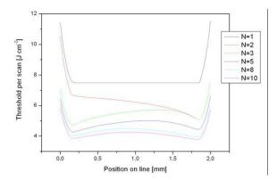
Figure 3. Local damage threshold for multiple scans, for a spot size of 288 μm top hat profile, and a scan speed of 100 mm/s (i.e. 100 times faster as in figure 2). N denotes the number of scans, where the scans where of alternating direction. Adopted from [6]
