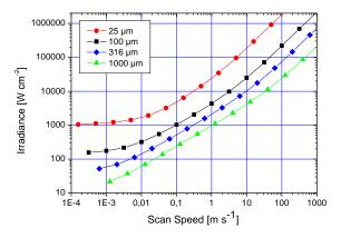
**Figure 4.** Calculated damage thresholds as function of scan speed for four different spot sizes for a Gaussian beam profile (1/e) for a single scan. Adopted from [6]
