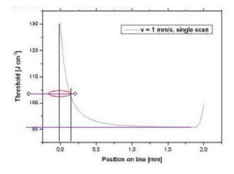
**Figure 2.** Local damage thresholds for a single scan with diameter of 288 μm top hat profile and a scanning speed of 1 mm/s and a scan length of 2 mm. Adopted from [6]
