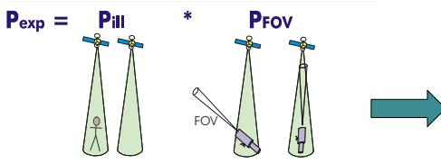
For ocular exposure to occur, the laser beam has to be incident on the location and the satellite has to be in the field of view.
