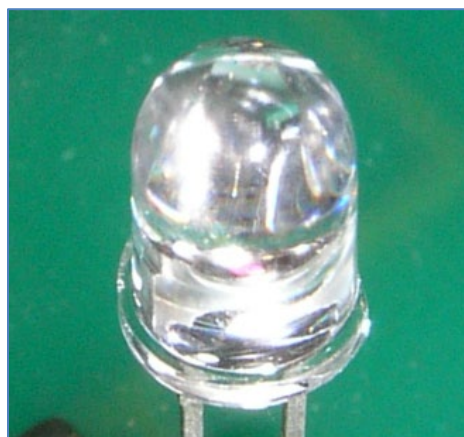
Figure 6. For this classic type of LED, the half-spherical top of the housing constitutes a lens.
