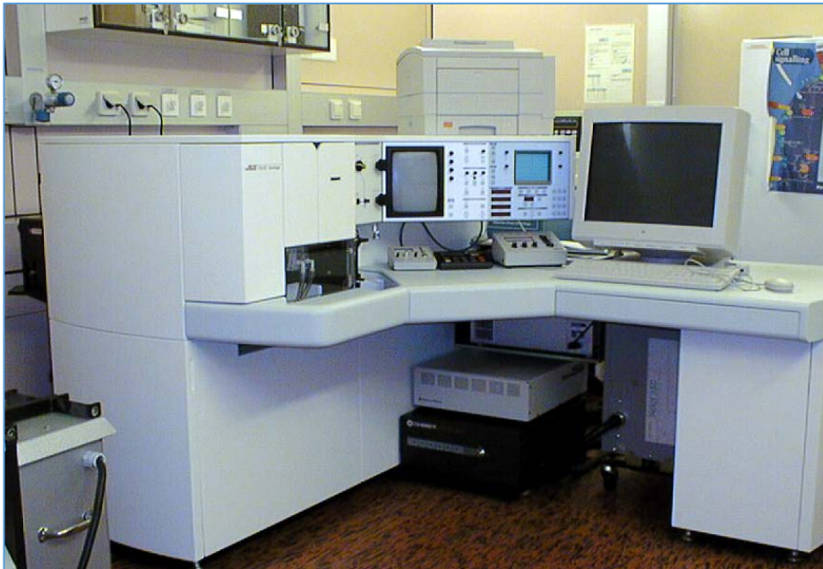
Figure 4 Cell sorters have to be classified as Class 3B or Class 4 when user procedures make it necessary to open the protective housing and change laser sources and align laser beams. This can still be considered as „safe“ product that complies with the requirements of A11:2021 and the LVD.
