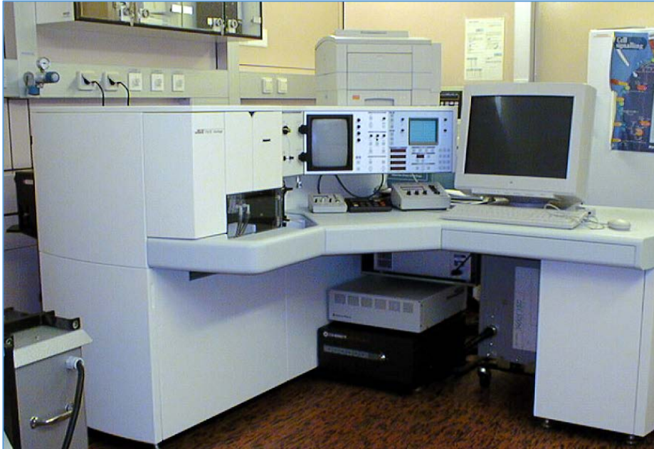
Figure 4 Cell sorters have to be classified as Class 3B or Class 4 when user procedures make it necessary to open the protective housing and change laser sources and align laser beams. This can still be considered as „safe“ product that complies with the requirements of A11:2021 and the LVD.
