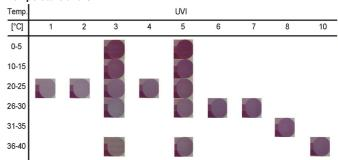
The matrix above shows that the ambient temperature has a stronger impact on the discoloration of the indicator field than the UVI. The following figure shows that the lower the ambient temperature the more intense is the discoloration at the same UVI. At high UVI ( $\geq 8$ ) and high temperatures ( $\geq 30^{\circ}\text{C}$ ) the colour of the indicator field does not correlate well with the UV exposure, as the colour of the indicator field gradually fades due to the increasing temperatures.
